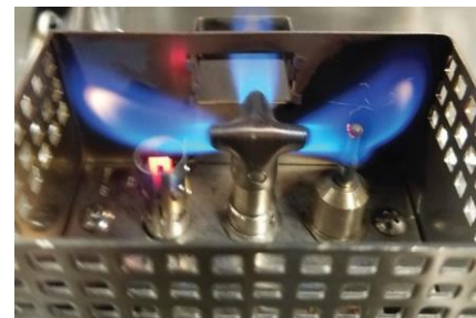
Figure 10.2 – Pilot flame coverage of thermocouple.
